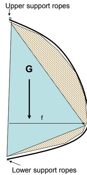
Fig. 24. Net deflection and self-weight of the net's belly. Figure according to [36].
