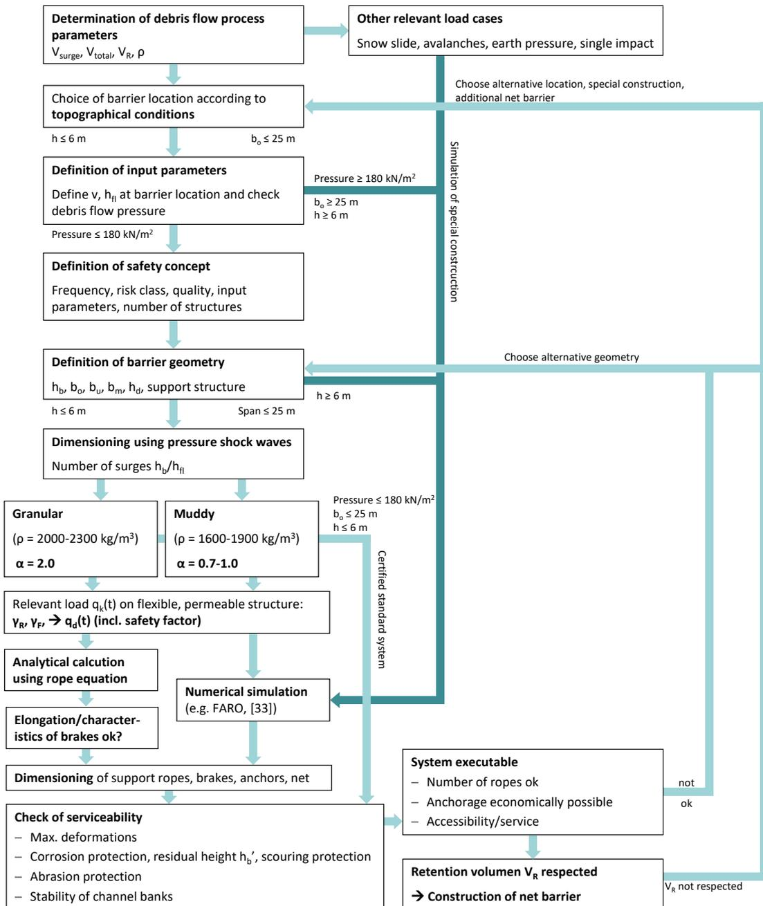
Fig. 18. Design flow chart for debris flow protection nets, according to [36].
